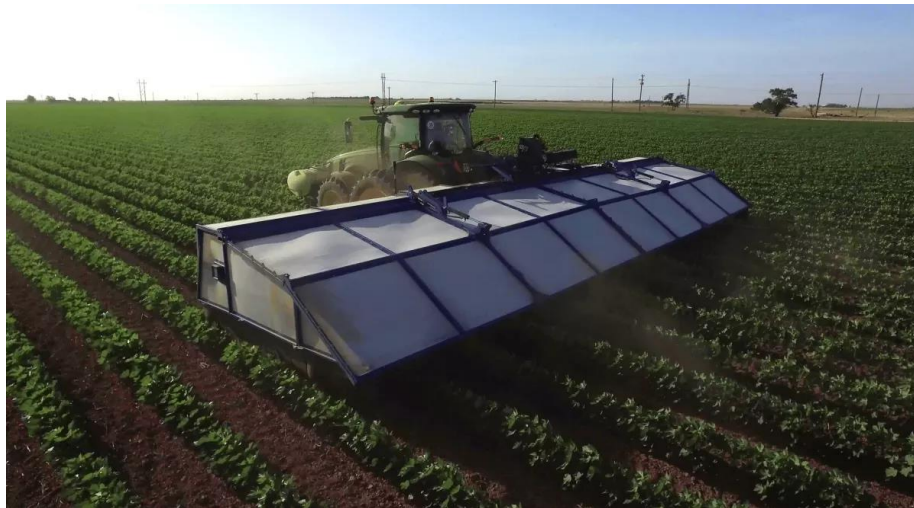
Figure 3.5. The See & Spray robot developed by Blue River Technologies [27]
