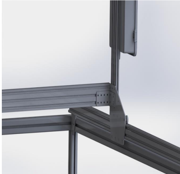
Figure 6.8. The y-axis was attached to the wheel bearing connector so that it could be lowered as much as was needed.
