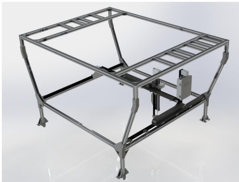
Figure 7.4. The final design of the frame
