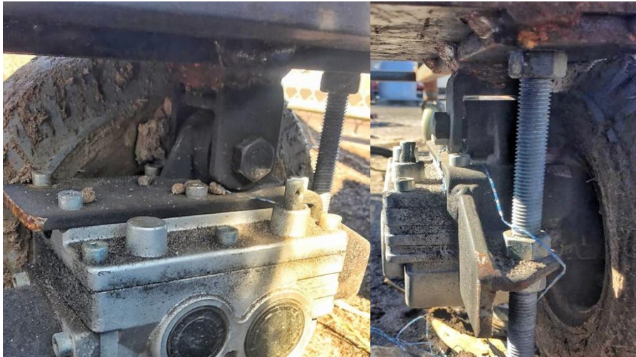
Figure 6.18. The two attachment points for the motor
