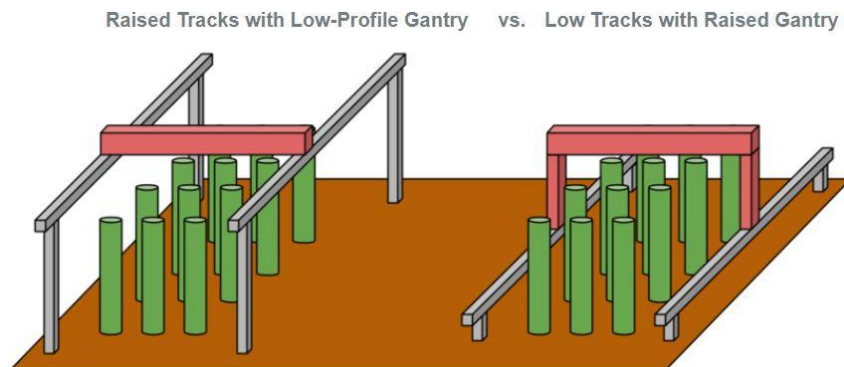
Figure 3.16. Raised tracks vs low tracks [34]
