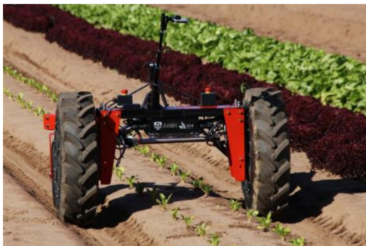
Figure 6.13. Digital Farmhand is a small robot, but it still uses the same type of tread pattern used on many bigger robots [57]
