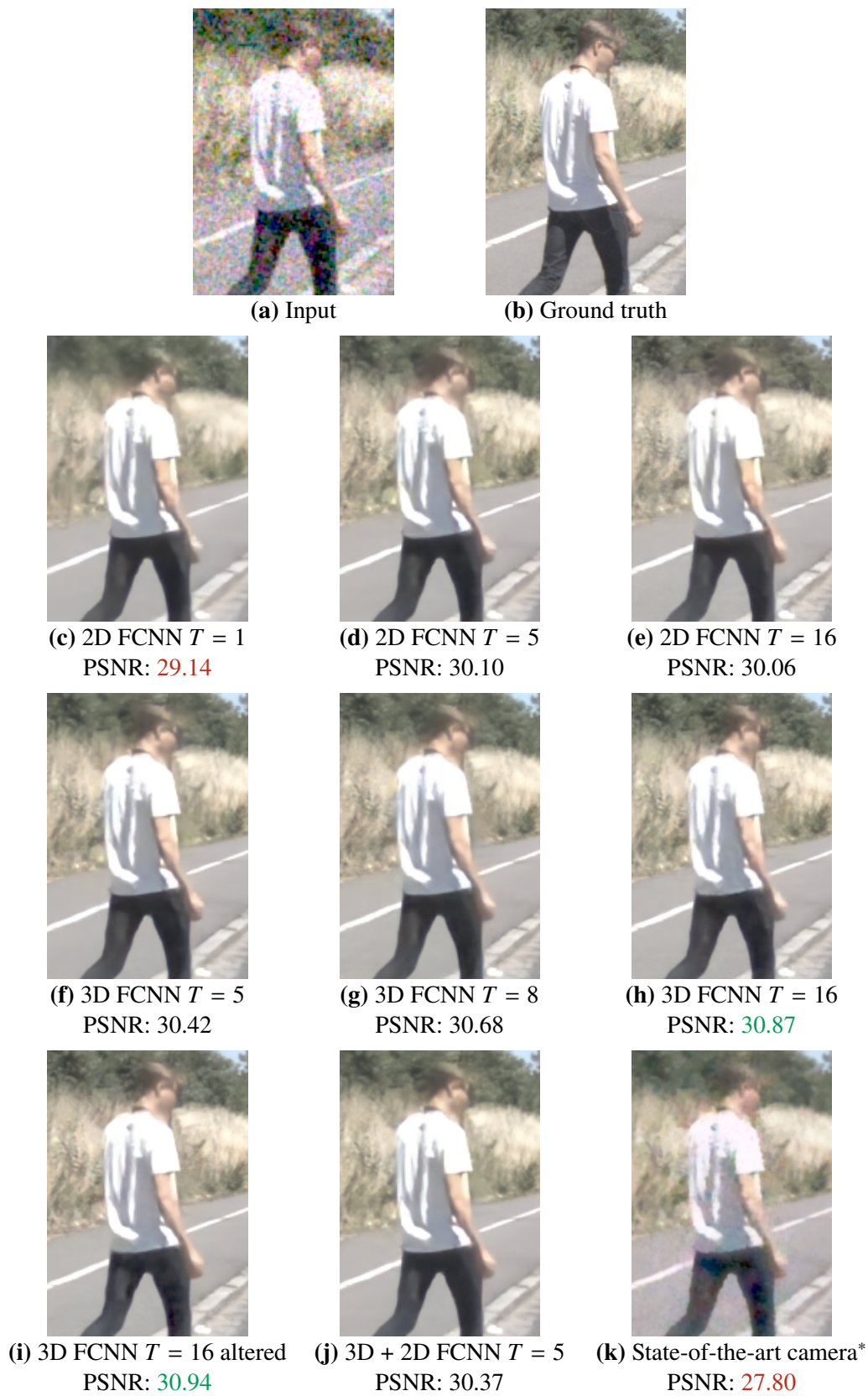
Figure 4.3: The performances when denoising a frame in a sequence with a person that is moving relatively slowly. Figure 4.3i refers to the network with P = 128 and 3 levels.
