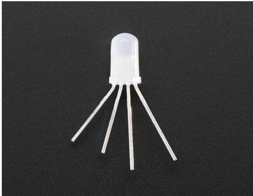
Figure 10. A NeoPixel, the LED pixel used (Adafruit, 2017).
