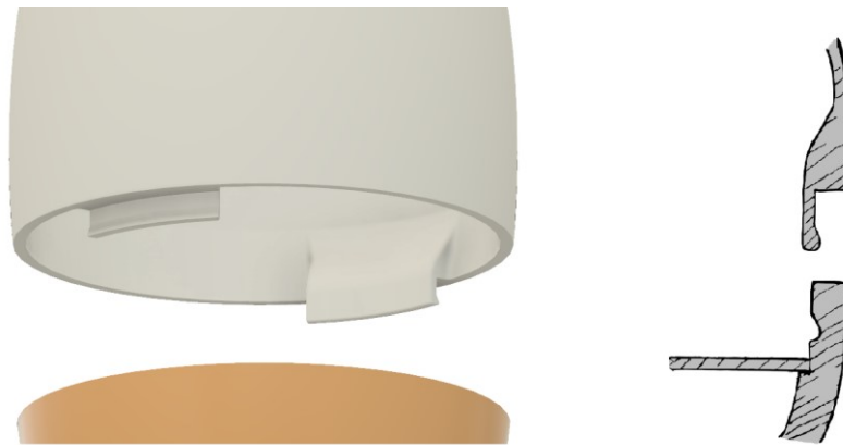
Figure 30. A 3D model and a cross-section of the chosen attachment mechanism.
