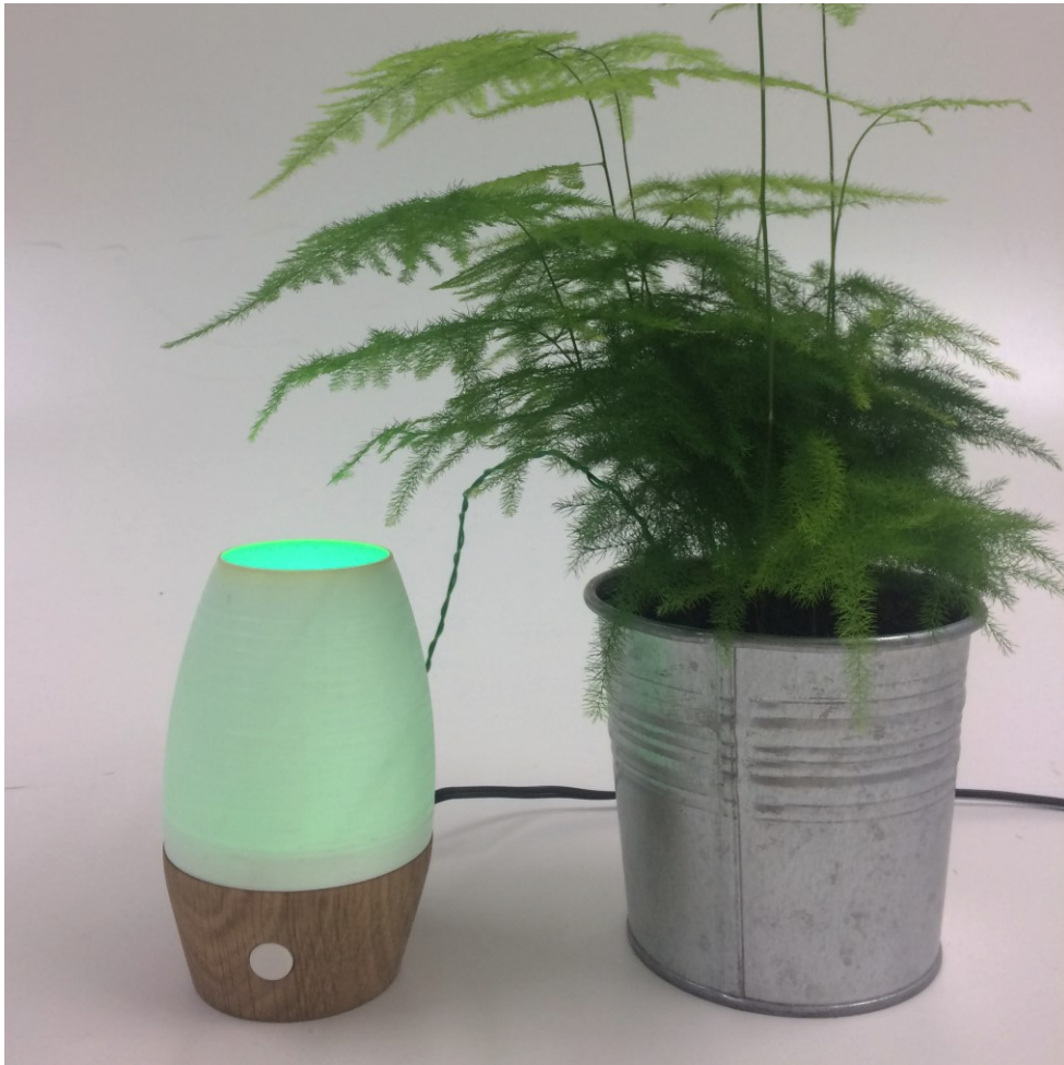
Figure 33. The prototype emitting a green light to indicate a high moisture level in the soil.
