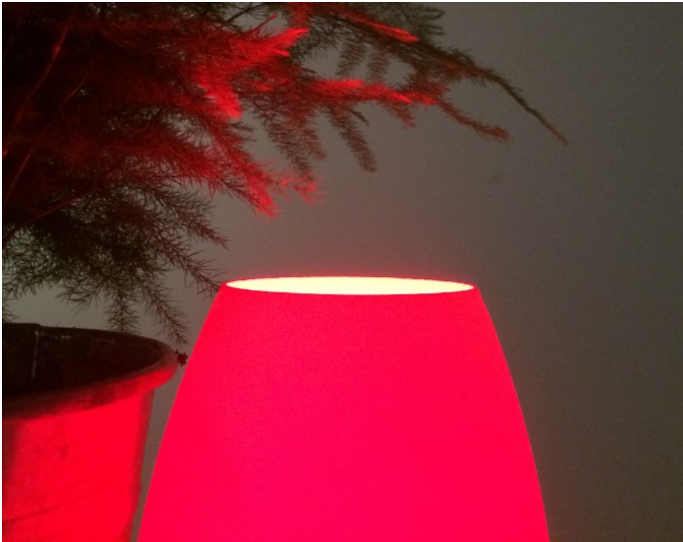
Figure 35. Red color indicating a low moisture value in the soil.
