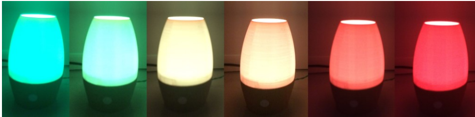
Figure 34. Colors emitted as the moisture level in the soil decreases.
