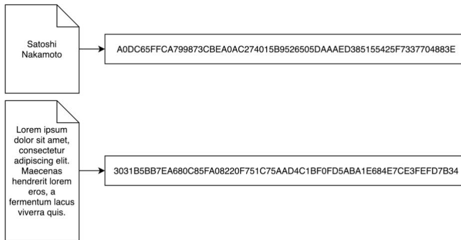
Figure 2. Two messages and their corresponding SHA-256 hash value. This figure was made by the author of this thesis.
