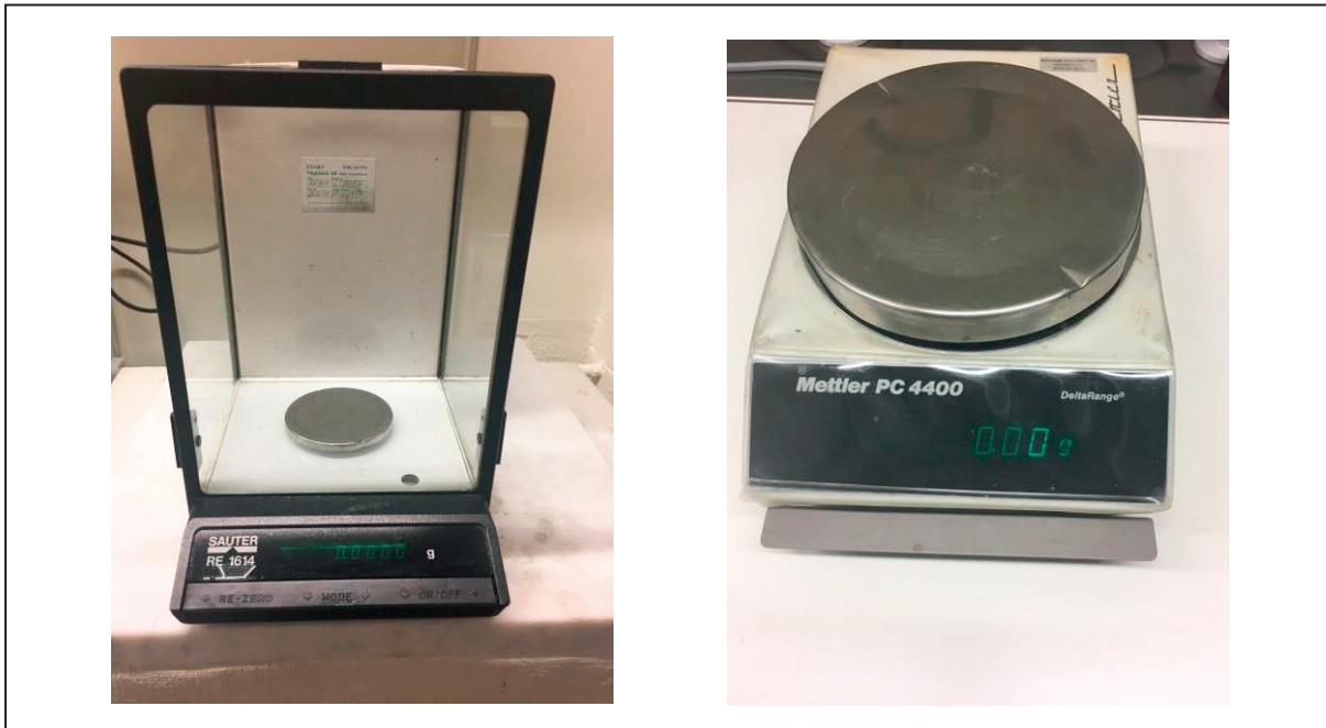
Figure A.0.4 The scales used for this study ( left side: 4 decimal scale, right side 2 decimal scale)
