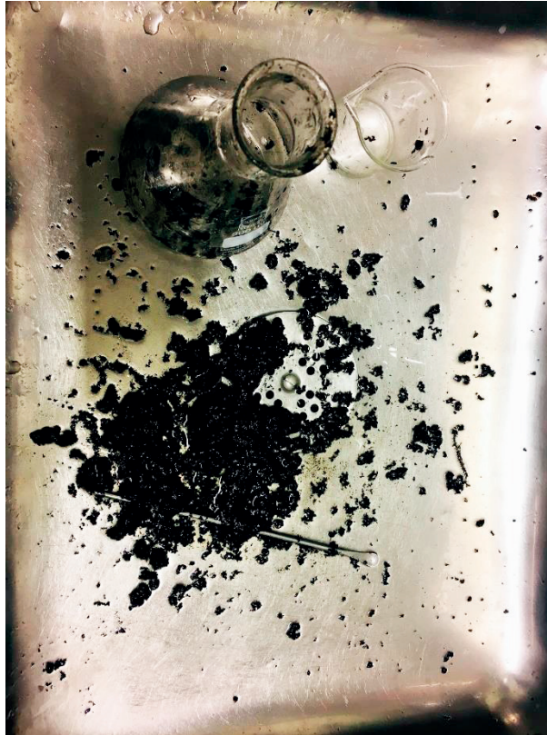
Figure 5.1 The state of the conditioned sludge for dose 8 g/kg DS sludge for the two polymer type.
