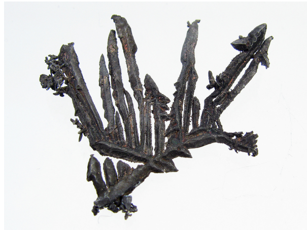
Figure 3: A dendritic crystal of silver as a mineral, the black colour comes from slightly oxidized silver [21].
