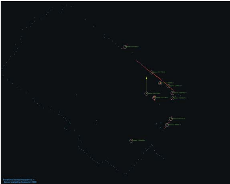
Figure 5.8: A screenshot of the author's implementation, showing a room scan. The yellow arrow marks the direction of the Sweep
