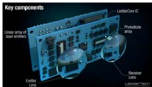
Figure 2.6: Solid state LiDAR with laser flash technique [12]
