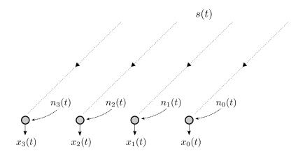
FIGURE 2.9: Anechoic signal model under far-field assumption.
