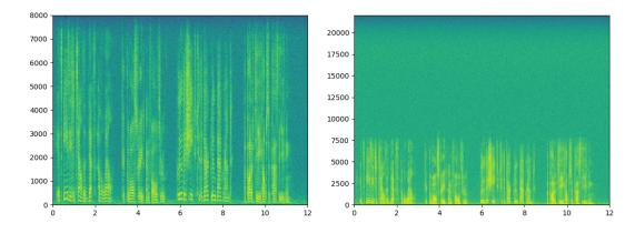
FIGURE 5.2: Spectrogram of clean SOI with  $F_s = 16$  kHz and 44.1 kHz respectively.
