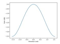
FIGURE 2.14: Frequency response with a frequency of 1000*Hz* for 16 microphones confined to a matrix, spaced with 21*cm* and 4.2*cm* respectively.
