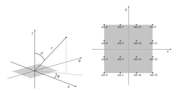
FIGURE 2.4: Orientation and enumeration of microphone array.
