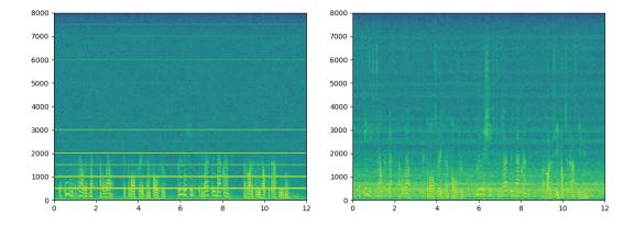
FIGURE 5.8: Spectrogram, before and after beamforming with MVDR respectively.
