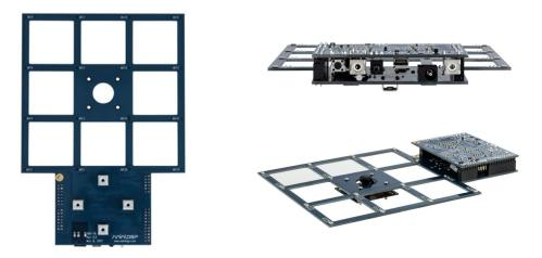
FIGURE 1.1: Microphone array used during the thesis.
