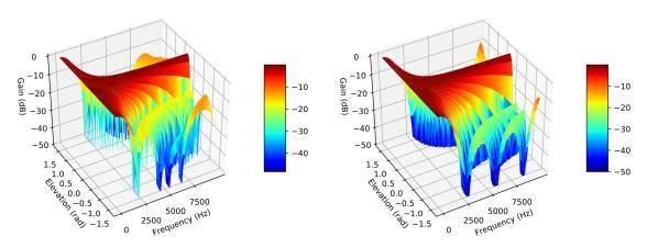
FIGURE 2.18: Frequency response for 16 microphones, spaced with 4.2 cm, with azimuth angle at 22.5° and 45° respectively.
