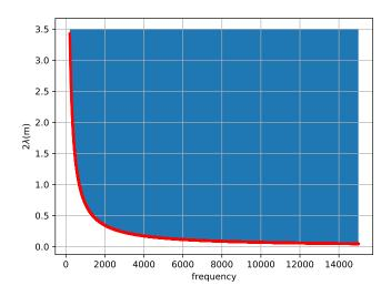
FIGURE 2.2: Far-field (blue region) and near-field (area under curve).
