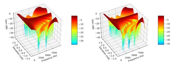
FIGURE 2.17: Frequency response for 9 and 16 microphones respectively confined to a square (matrix), spaced with 4.2 cm.
