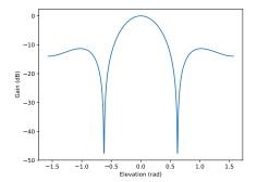
FIGURE 2.15: Frequency response with a frequency of 3500 for 16 microphones confined to a matrix, spaced with 21 cm and 4.2 cm respectively.
