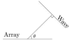
FIGURE 2.10: Angle of incident.
