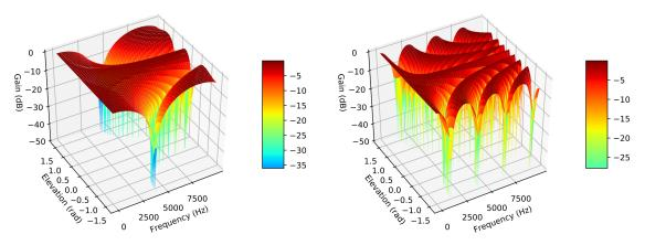
FIGURE 2.16: Frequency response for 4 microphones confined to a square, spaced with 4.2 cm and 12.6 cm respectively.
