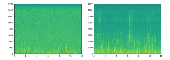
FIGURE 5.7: Spectrogram, before and after beamforming with MVDR respectively.
