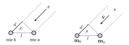
FIGURE 2.6: Different representations of a simple microphone array and a propagating source.
