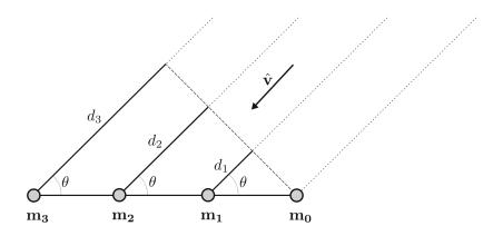
FIGURE 2.7: Microphone array - positions and propagation.
