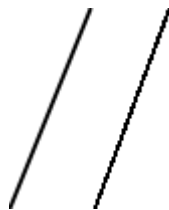
Figure 3.4: Ground Truth image of a Line versus its Aliased Approximation.
