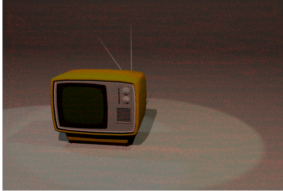
Figure 3.6: Example of Precision class with a sporadic error. For illustration purposes, a semi-transparent one channel BDI is layered over the reference image (as most precision errors of this sort are not visible to the human eye) with red pixels to represent errors. In this case, the errors are appearing randomly across the image.
