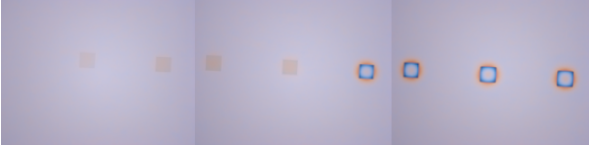
Figure 25: Optical microscopy image of the results from the imprinting with the IPS intermediate stamp. The squares are the arrays of holes. The EBL exposure dose for each square is different, with the highest dose farthest to the left, and the lowest dose farthest to the right.
