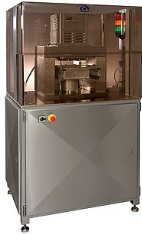
Figure 4: The Obducat nanoimprint lithography system used in Lund Nano Lab. 25
