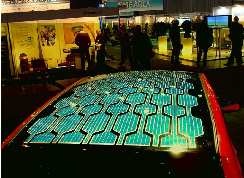
Figure 7.5 Flexible PV cells on a car roof.
