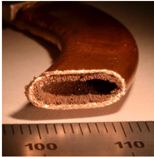
Figure 4.1 An intersection of a heat pipe.
