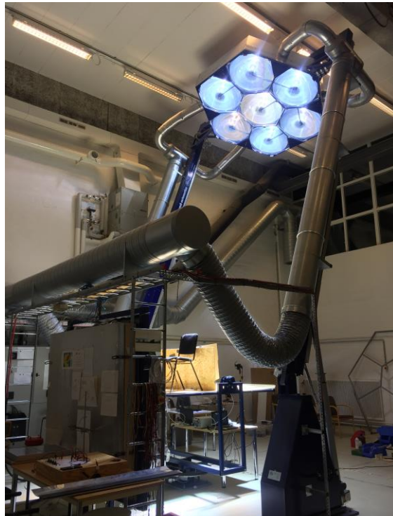
Figure 9.17 Solar simulation lamp in LTH solar laboratory.
