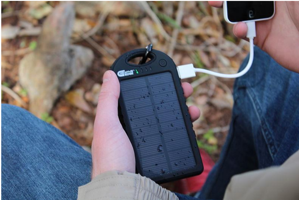
Figure 7.2 PV cell phone charger.
