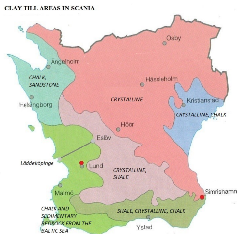
Figure 3.4. Areas of clay tills in Scania. Study sites are marked with red circles. The cross-section between Lötterköpinge and Eslöv cities is marked with a grey line. Modified from Ekström (1936).
