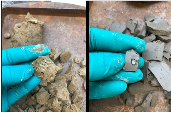
Figure 3.9. A sandy, silty brown clay till (left) and a clay-rich, grey clay till (right) with clasts from Simrishamn site. Photo by the author, 2018
