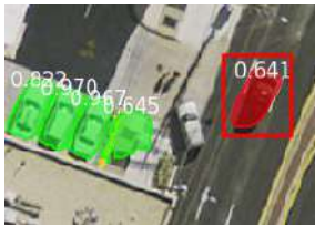
Figure 5.1: Post-processing idea of removing parking spaces that have no neighbours.
