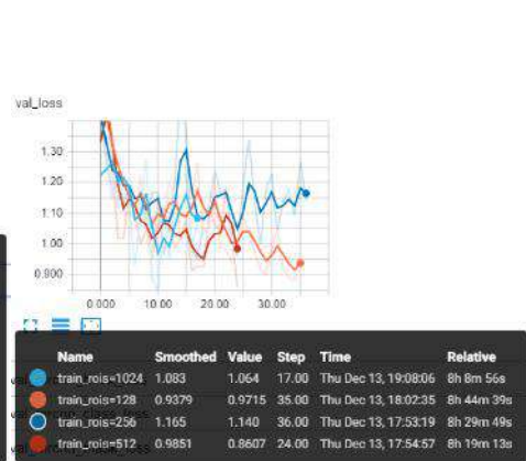
Figure A.10: Tensorboard graph - TRAIN_ROIS_PER_IMAGE
