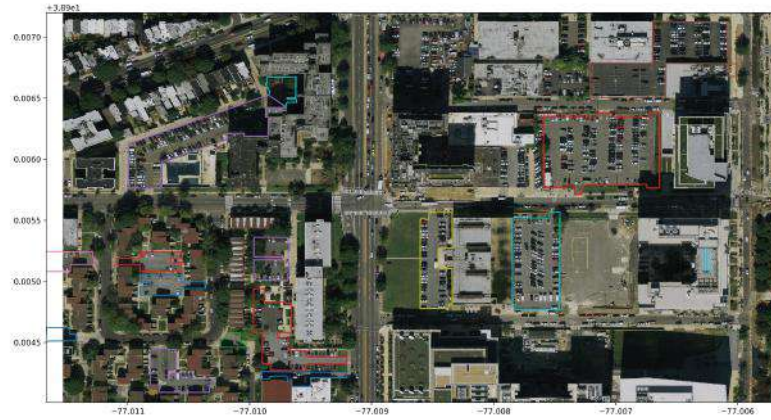
Figure 3.4: OSM data overlaid on a test image. The drawn polygons on the image represent individual parking lots.
