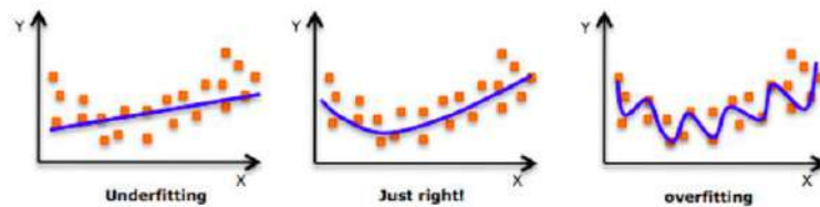
Figure 2.5: A comparison between underfitting and overfitting models. The blue lines are the outputs from the model, and the red dots are ground truth samples, by Shubham Jain [4]
