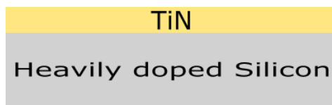
Figure 3.2: Schematic of the sample after TiN BE sputtering.
