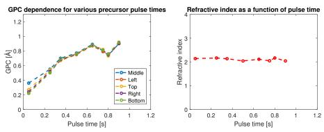
(a) GPC dependence on pulse time for dif- (b) Refractive index dependence on pulse ferent placements in the deposition time for  $\lambda=600nm$ . chamber.
