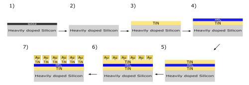
Figure 3.8: Schematic of the entire sample process step by step.
