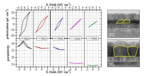
**Figure 2.8:** P-V and C-V hysteresis curves for a thickness series of pure  $HfO_2$  thin films crystallized in the precence of a PVD-TiN top electrode (left). TEM micrograph comparison of the 6nm and 20nm  $HfO_2$  films [4].
