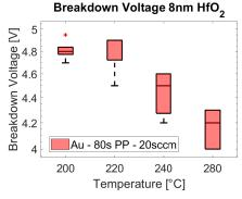
(c) Breakdown voltage for xsmall structure for increasing deposition temperature.
