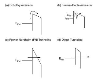
**Figure 2.16:** Tunneling mechanisms of insulators schematically displayed. Image taken from [6].
