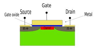
Figure 2.1: Schematic of an n-type MOSFET.
