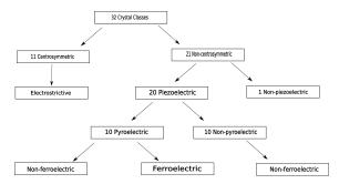
Figure 2.2: Arrangement of the 32 crystal classes.
