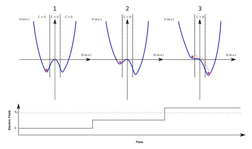
Figure 2.4: 1 Energy landscape U of a ferroelectric material in the absence of an electric field. 2 Landscape change in presence of an electric field smaller than the coercive field  $E_c$ . 3 Evolution of energy landscape when an electric field greater than  $E_c$  is applied and the polarization passes trough the state of negative capacitance.
