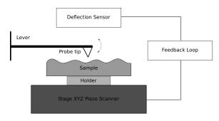
**Figure 2.21:** Schematic of experimental setup for an atomic force microscope.
