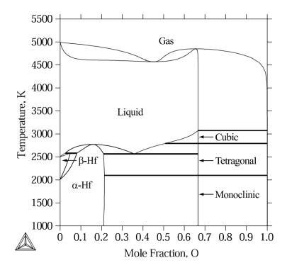
Figure 2.7: Binary diagram of Hf-O [3].
