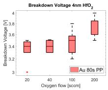
(c) Breakdown voltage for xsmall structure at increasing oxygen flow.
