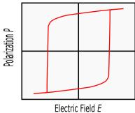
**Figure 2.13:** Hysteresis of a ferroelectric material.
