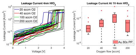
(a) J-V characteristics for xsmall structure (b) Leakage current at 1V for xsmall structure from for varying oxygen flow.
