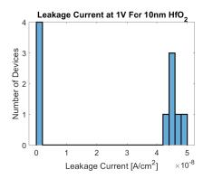
(a) I-V characteristics for xsmall structure (b) Leakage current at 1V for xsmall structor for optimized sample.
