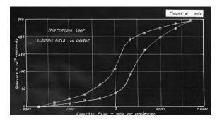
Figure 2.3: First hysteresis curve of a ferroelectric material [1].
