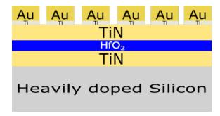
Figure 3.5: Schematic of the sample after evaporation.
