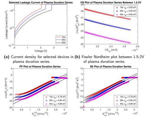
(c) Poole Frenkel plot of plasma duration (d) Schottky plot of plasma duration series series with a linear approximation at with a linear approximation at 1.5-2V.
