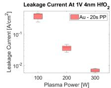
(a) J-V characteristics for xsmall structure (b) Leakage current at 1V for xsmall structure at increasing plasma power.
