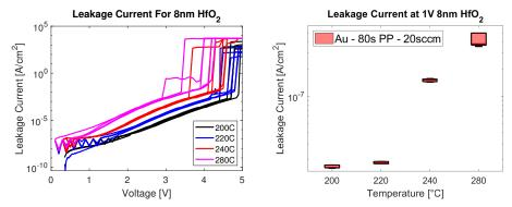
(a) J-V characteristics for xsmall structure (b) Leakage current at 1V for xsmall structure for varying deposition temperature. ture for increasing deposition temperature.
