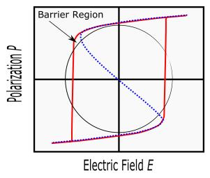
**Figure 2.14:** Schematic of Hysteresis curve for a ferroelectric material where the red curve denoted the measured, turquoise the accurate polarization where the negative differential capacitance is present in the barrier region.
