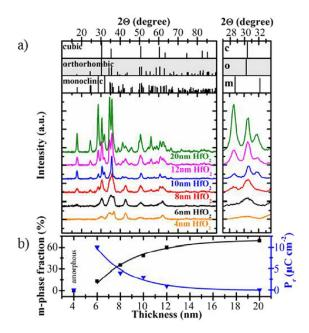
Figure 2.9: (a) GIXRD data for a thickness series of pure  $HfO_2$  crystallized in the presence of a PVD-TiN top electrode. The inset shows an enlargement of the prominent reflexes for the monoclinic, orthorhombic and cubic phase structure, which were used for the calculation of the monoclinic phase fraction. (b) Calculated monoclinic phase fraction and corresponding values of remanent polarization  $P_r$  as a function of film thickness. [4].
