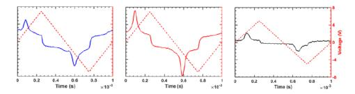
Figure 5.14: I-T curves of ferroelectric oxides by Karine Florent. Image Taken from [8]
