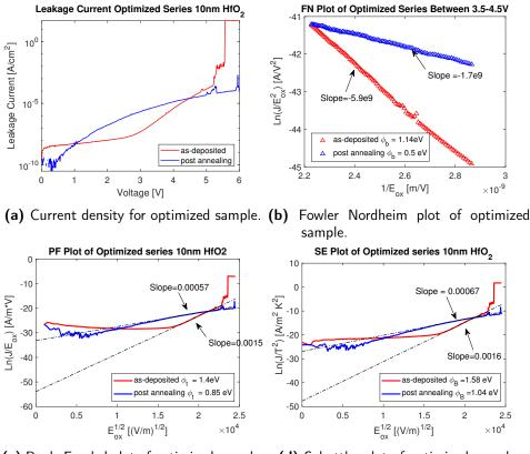
(c) Poole Frenkel plot of optimized sample. (d) Schottky plot of optimized sample.
