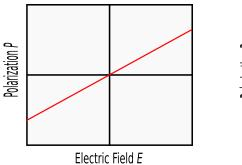
**Figure 2.12:** P-E curve of a ideal capacitor.
