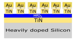
Figure 3.7: Schematic of the sample after TiN etching.
