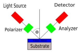
**Figure 2.20:** Schematic of experimental setup for ellipsometry measurements.
