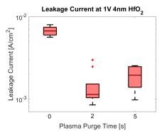
(a) J-V characteristics for xsmall structure (b) Leakage current at 1V for xsmall structure for varying plasma purge duration.
