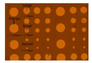
**Figure 3.6:** Optical spectroscopy image of fabricated sample after metal deposition.
