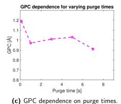
**Figure 5.1:** Calibration of GPC for TEMAHf source in Fiji F200 ALD.
