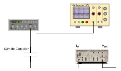
**Figure 4.1:** Measurement setup for P-E.
