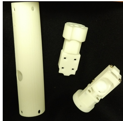
Figure 4.5: The 3D printed outer cylinder next to the top part eventually holding the fiber and the bottom part (here with only one horizontal attocube).
