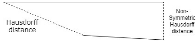
Figure 4.1: Difference between Hausdorff distance and Non-symmetrical Hausdorff distance, when line length is large. The non-symmetric Hausdorff distance is computed from the shorter line to the longer line.
