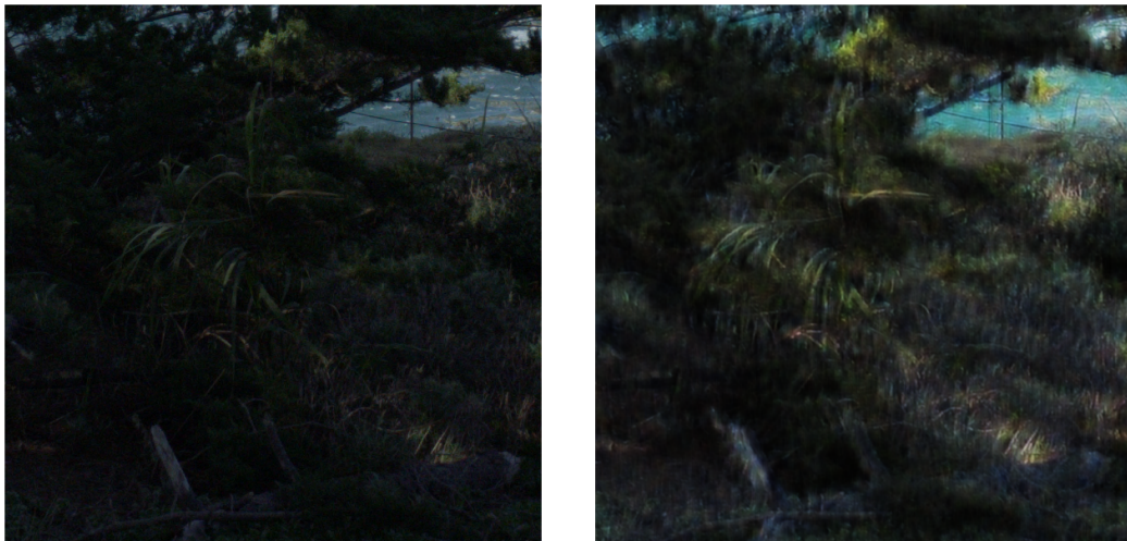
Figure 6.3: Blurry edges introduced by the network. Left image is the input image, right image is generated by the multi-image network.
