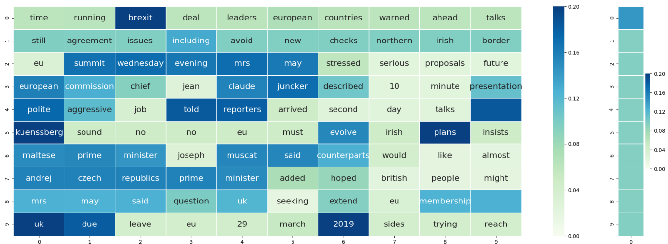
Figure 4.2: The attention weights visualized for the 3HAN model. The sentence attention is visualized in the table to the right.
