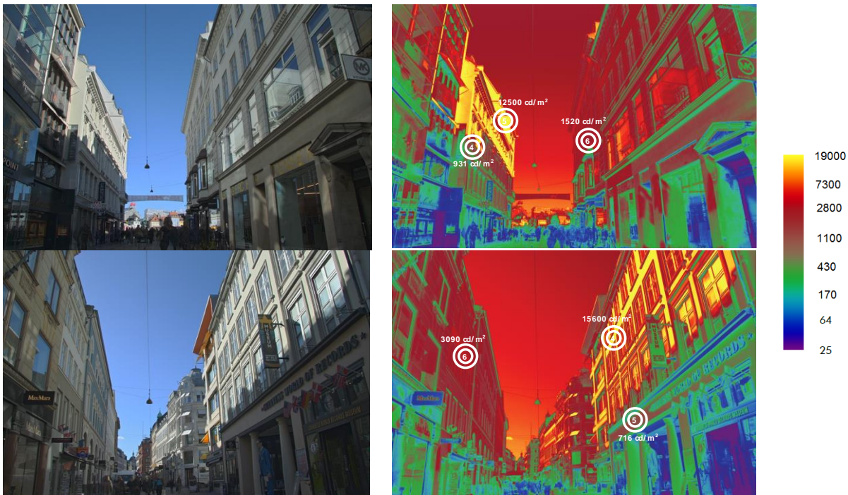
Figure 28 Canyon "O". Top – A', bottom – A''. Left side – HDR photos, right side – false color diagrams and points of measurements.
