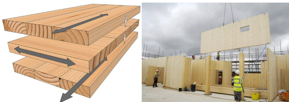
Figure 10.3: Solid sawn lumber placed orthogonally placed.(Reid Middleton 2017). CLT panel (Big Red Dog 2017).
