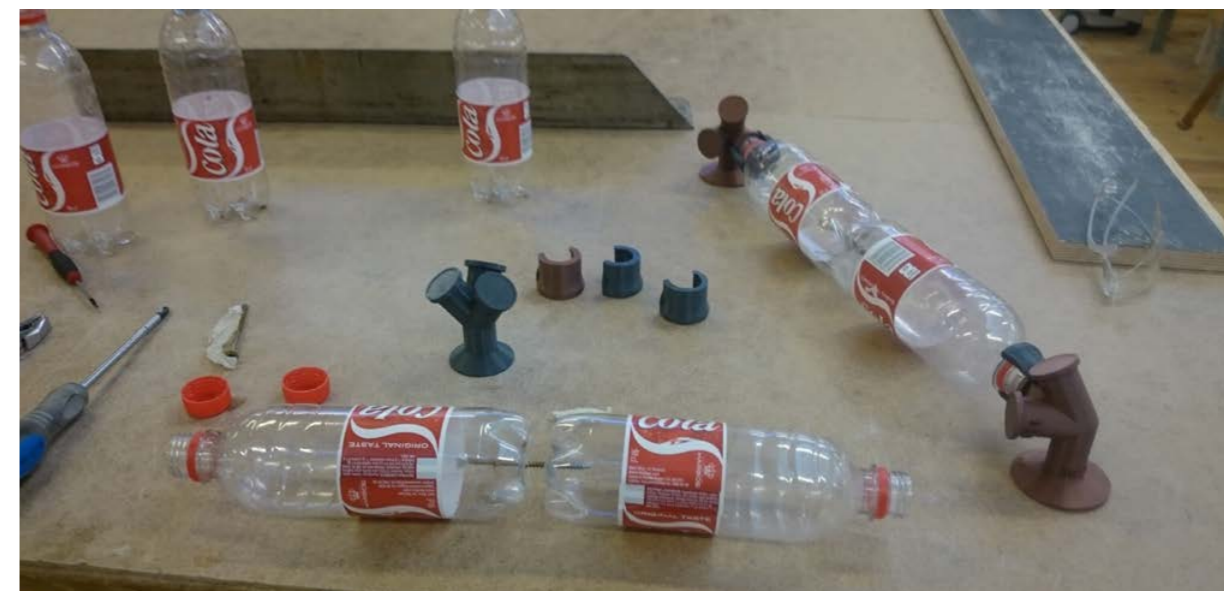
Figure 120. Building the truss beams
