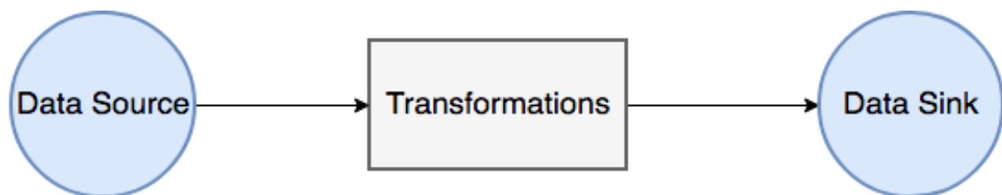
Figure 1.3: Image describing a basic stream program in Flink, where the arrows are the intermediate streams and the blocks are the operators.
