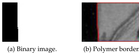
FIGURE 4.6: The border of the polymer against an unilluminated background. The left subfigure shows the binary image resulting from the thresholding operation and the right subfigure shows the border as a red line consisting of the outermost pixels of the connected component corresponding to the polymer.
