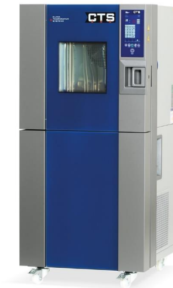
Figure 11: Photograph of CTS climate chamber used in the present investigation.
