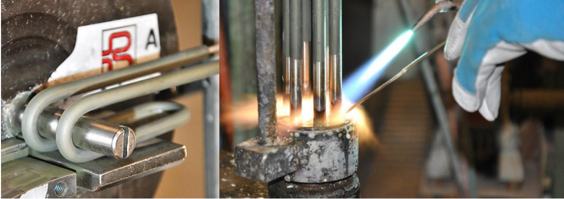
Figure 6: Bending of a tubular heating element (left) and brazing (right)
