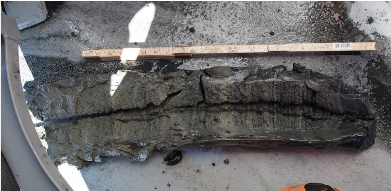
Fig. 3 Laminated sediment collected at the site Gp2. 0-20 cm has distinct laminated layers. Photo credit: Kotaro Hirose 2017
