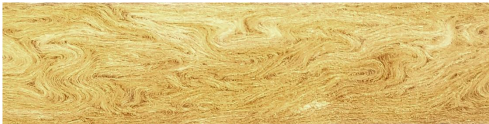
Figure 3.2 Cross section crimped glass wool.
