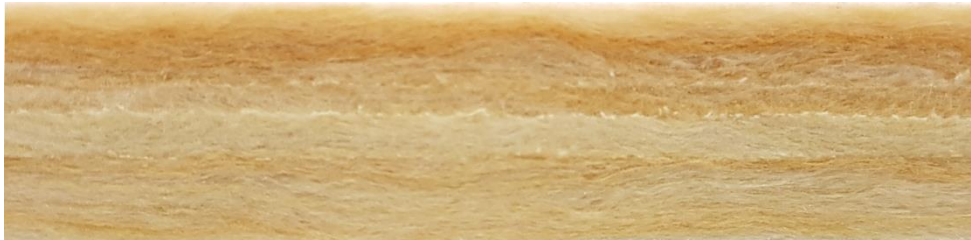
Figure 5.7 Close-up of the unpainted edge for prototype “GB, 4”, ca 30 mm thick
