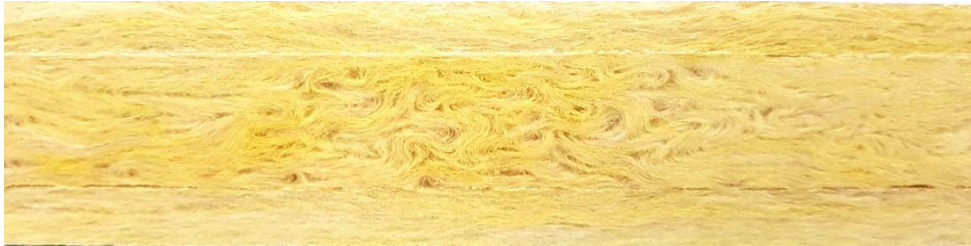
Figure 5.8 Close-up of the unpainted edge for prototype “Crimped Sandwich”, ca 40 mm thick
