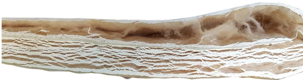
Figure 3.12 Acoustic board after being subjected to a warm and humid environment for a prolonged period of time.
