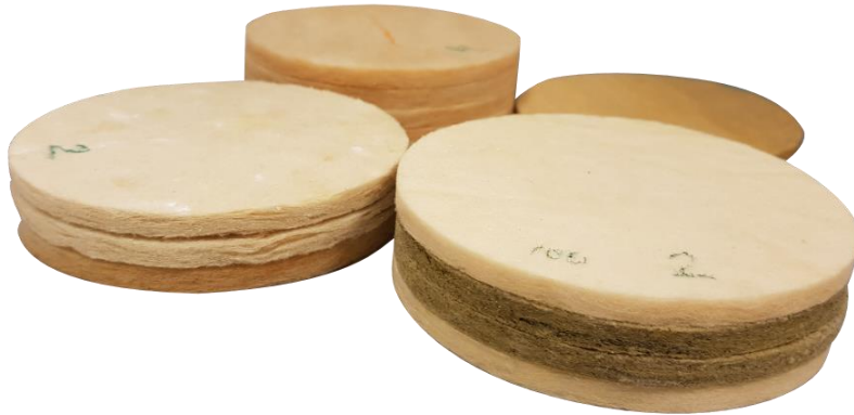
Figure 5.9 Combinations of 5 mm layers prepared for AFR-testing
