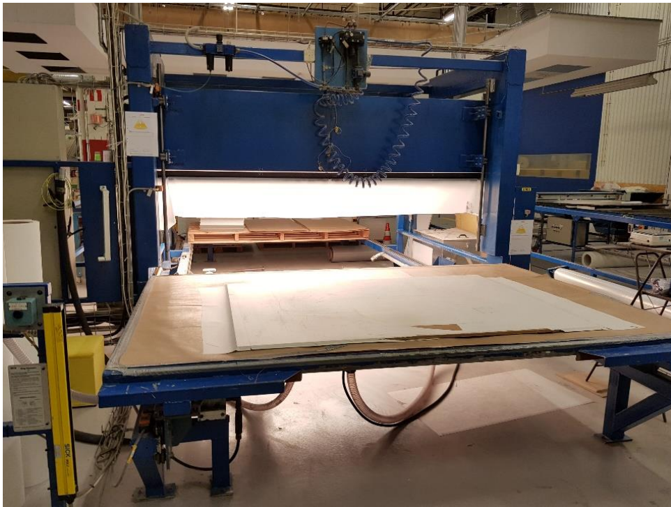
Figure 5.2 Small scale lamination machine used for custom made products.
