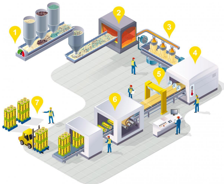
Figure 3.1 Schematic of the manufacturing process for glass wool. [5]
