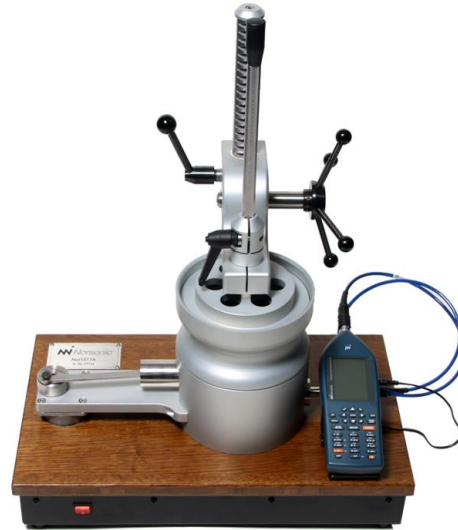
Figure 3.6 T.t.l: Die punch used to get the appropriate size of the sample. T.t.r: AFR measuring equipment Nor1517A from Norsonic. Image taken from [18]
