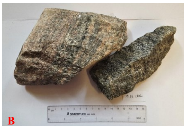
Fig. 12. (a) Close-up of the Hälltorp migmatite at locality 9.1 in the Median Segment, which sample MISE1816 belongs to. (b) The left hand-specimen represents subsample MISE1816c leucosome and the right hand-specimen represents subsample MISE1816c melanosome.
