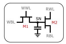
Figure 4.3: 2T NMOS eDRAM Gain Cell
