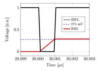
Figure 6.4: Read process for low level stored
