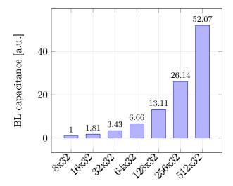
Figure 6.6: Bitline parasitic capacitance dependency with macro size
