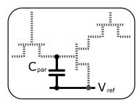
Figure 2.2: Generic DRAM cell with storing parasitic capacitance
