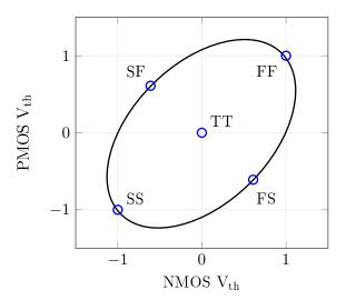
Figure 3.1: Process corners distribution
