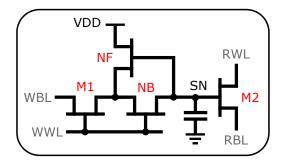
Figure 4.4: 4T NMOS eDRAM Gain Cell
