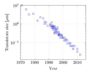
Figure 1.1: Technology scaling in the last 40 years [6]
