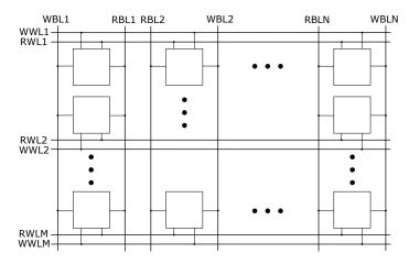
Figure 2.4: Matrix of bitcells in an eDRAM macro with the size of MxN
