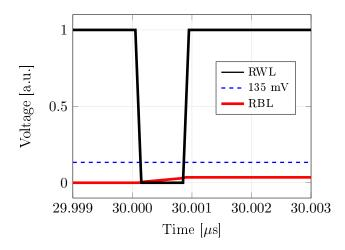
Figure 6.5: Read process for high level stored
