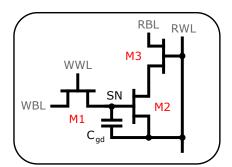
Figure 4.2: 3T NMOS eDRAM Gain Cell
