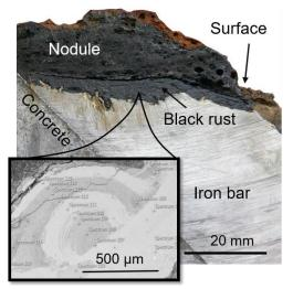
The black rust has replaced the upper most part of the iron bar and in the transition pit corrosion have started to breaking down the iron further. A nodule covers the top like a lid and prevents oxygen from reaching the corrosion area. With higher magnification the cyclic pattern can be seen.
