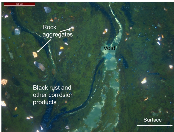
Fig. 6.8. Photomicrograph is taken in xpl with the darkfield mode enabled. This microdomain is situated a few millimeters further towards the surface (arrow pointing the right direction) of this sample, compared to Fig. 6.7. Black rust is seen in thinner bands within another corrosion product. In situ rock aggregates are left from the concrete material. The scale bar in the upper left corner is 500 µm.
