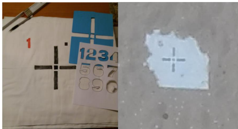
Figure 9. The artificial GCP, at the preparation time and from one of the flights.
