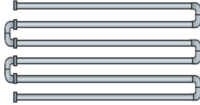
Figure 2.2. Holding tube going in a zig-zag pattern [1]
