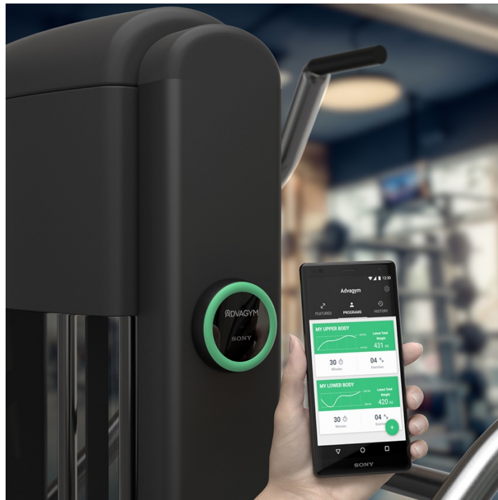
Figure 8, illustration of puck placement on a machine exercise, image courtesy of Advagym.
