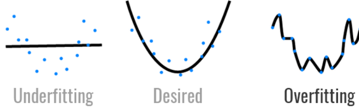
Figure 3.2: A schematic representation of underfitting (left) and overfitting (right) compared to the desired curve (middle) when fitting a parabolic curve to data points. Image from [26].
