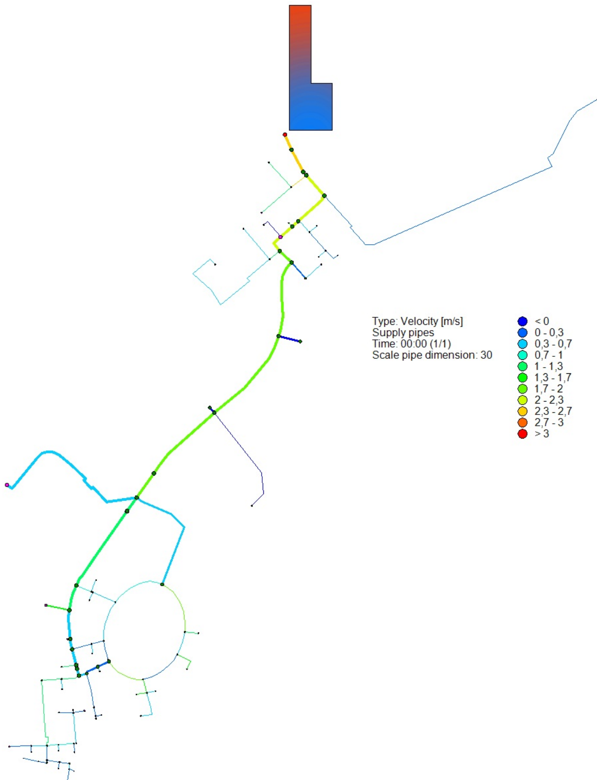
Figure 19: NetSim simulation of velocity with the projected heat demand in 2035.
