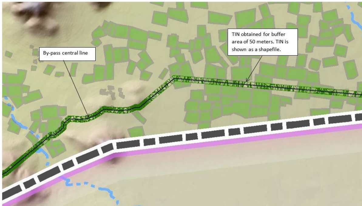
Figure 29. Example of created TIN datasets as a polygon shapefile imported into Novapoint (example shows part of a by-pass for an environmental theme)
