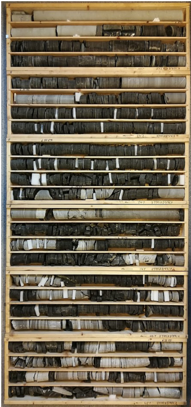
Fig. 1. The Alum Shale Formation in the Kinnekulle drill core displayed. The lowermost part of the formation are at the top of the picture, where also 1,5 m of the underlying lower Cambrian sandstone can be seen. Simplified; the black areas are organic-rich black shale and the grey areas are bituminous limestone.
