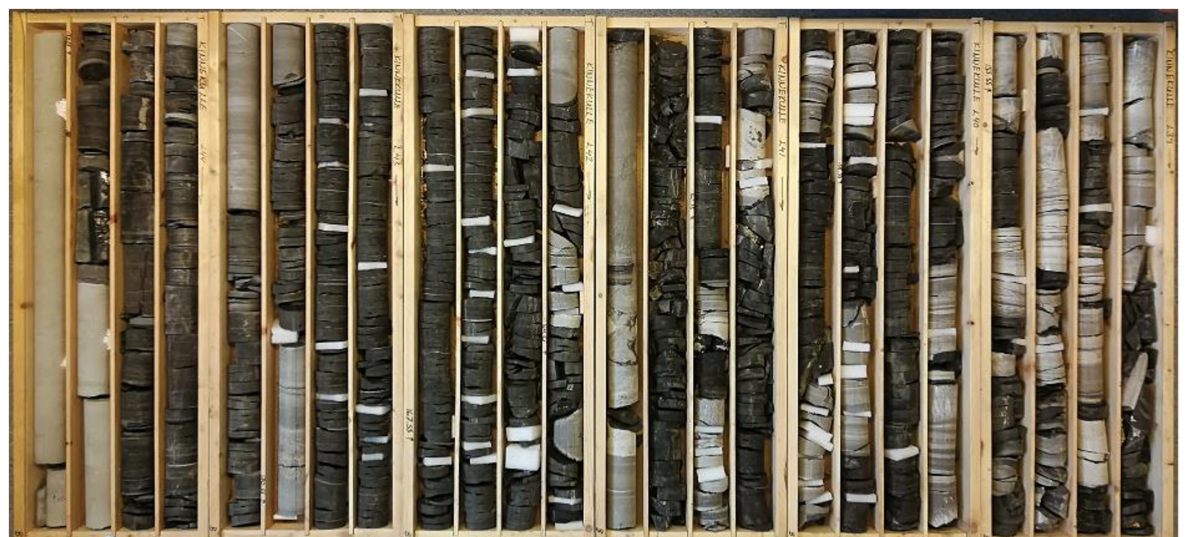
The Alum Shale Formation in the Kinnekulle drill core (recovered 2016 M. Calner, Department of Geology, LU) displayed. The lowermost part of the formation are to the left, where also 1,5 m of the underlying lower Cambrian sandstone can be seen. Simplified; the black areas are organic-rich black shale and the grey areas are bituminous limestone
