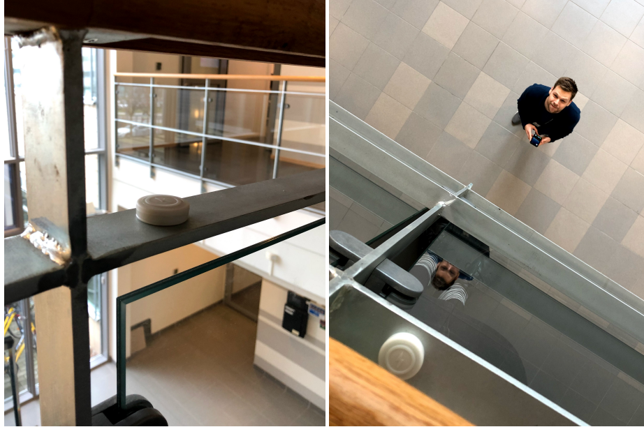
Figure 7.2: The test setting for the BLE beacon performance test carried out with a ceiling height of four and a half meters.
