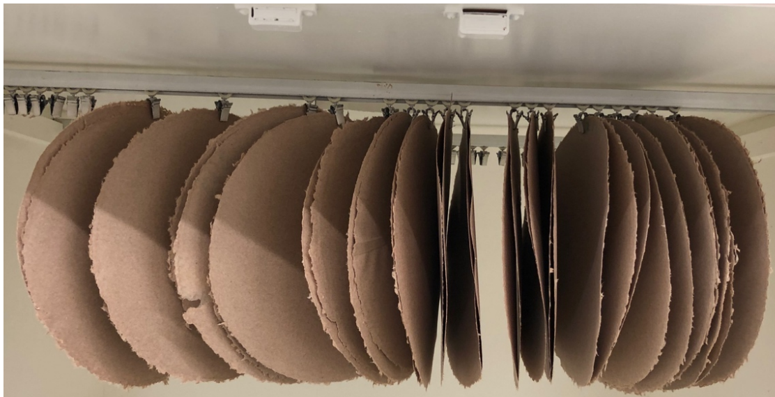
Figure 3.11. The sheets of paper made from recycled pulp being conditioned at 23 °C and 50% RH.
