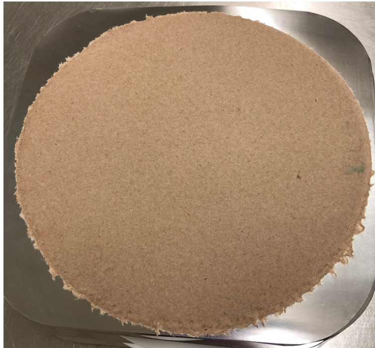
Figure 3.10. Sheet of paper made from recycled pulp. Seen on top of a pile with other sheets after being pressed at 0.55 MPa.
