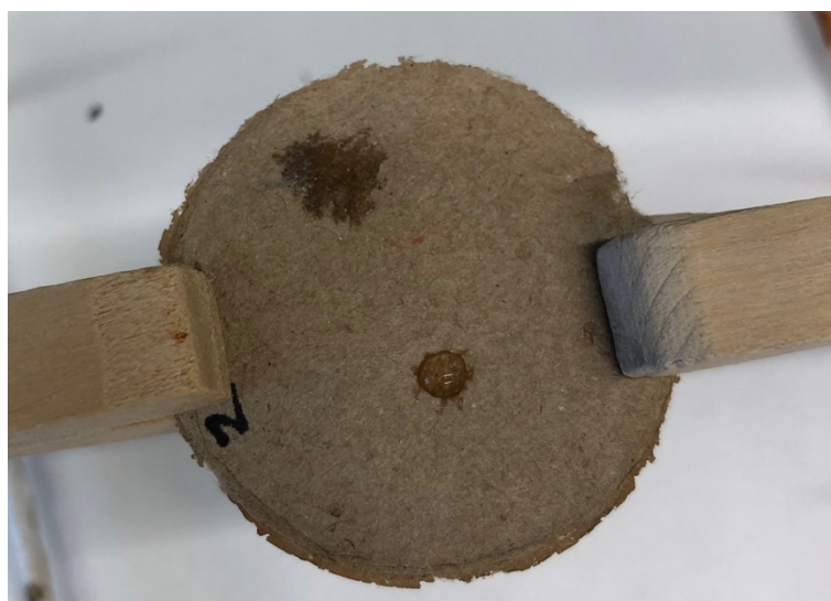
Figure 3.13. Drop test performed on paper made from homemade pulp. The top drop has already been absorbed and the bottom drop has just been applied.
