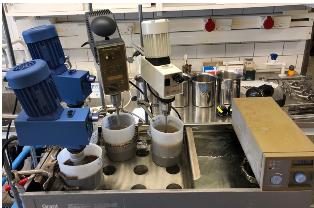
Figure 3.8. Experimental setup for the experiments with the papermill pulp.
