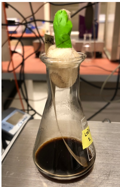
Figure 3.6. Setup of the paper treatment experiments. Part of the paper was in contact with the lignin solution and part of it never came in contact with it.
