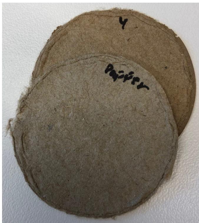
Figure 3.7. Papers from homemade pulp. The one on top has not been treated with anything, and the one below was treated with lignin and enzyme.
