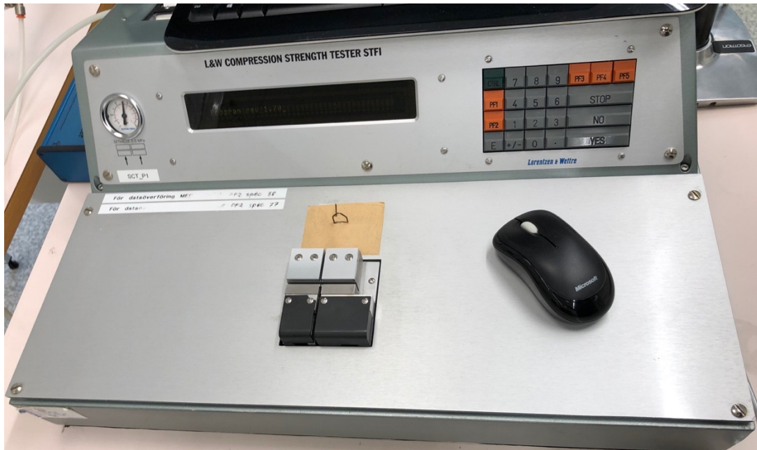
Figure 3.18. Equipment used for the compression strength tests.
