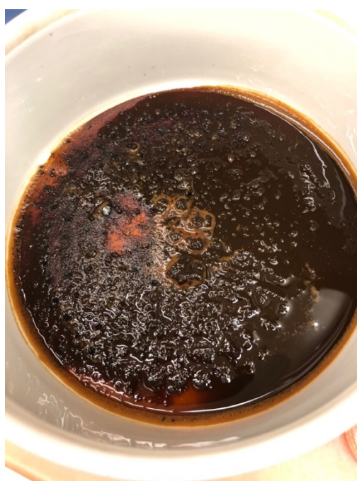
Figure 3.2. Filter cake of precipitated lignin.
