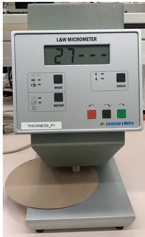
Figure 3.14. Apparatus measuring the thickness of the paper samples.
