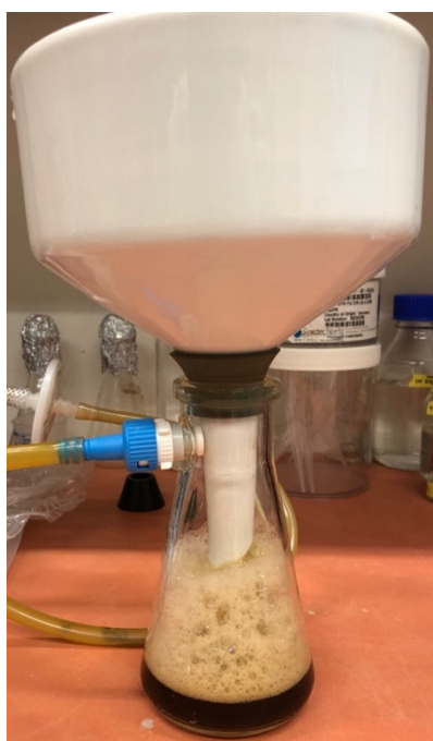
Figure 3.1. Foaming occurred when the lignin was filtrated.
