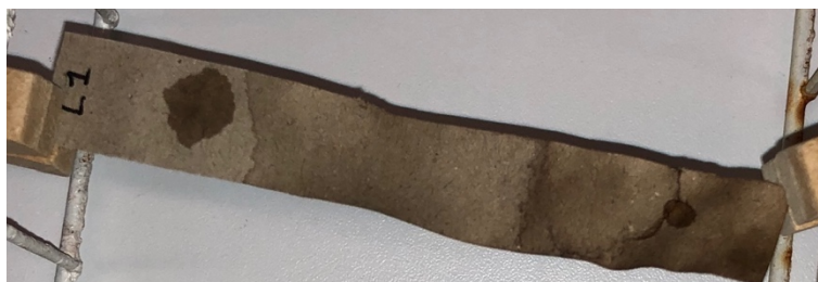
Figure 3.12. Drop test performed on treated paper. The left drop is on an untreated area, and the right is on the part of paper dipped in the lignin solution.
