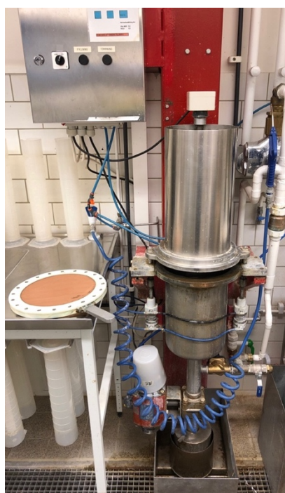
Figure 3.9. Sheet former used for forming sheets. Copper wire used to collect the pulp seen in the right corner.
