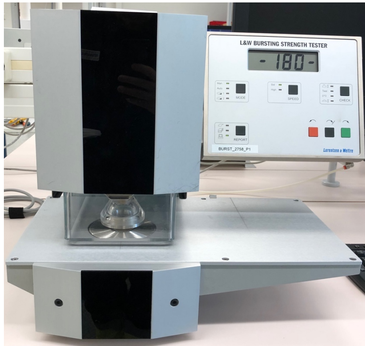
Figure 3.17. Equipment used for the bursting strength tests.
