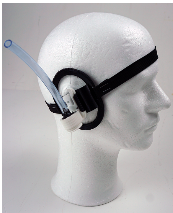
Figure 5.26: 3D print of strap and ear attachment, including TSI
