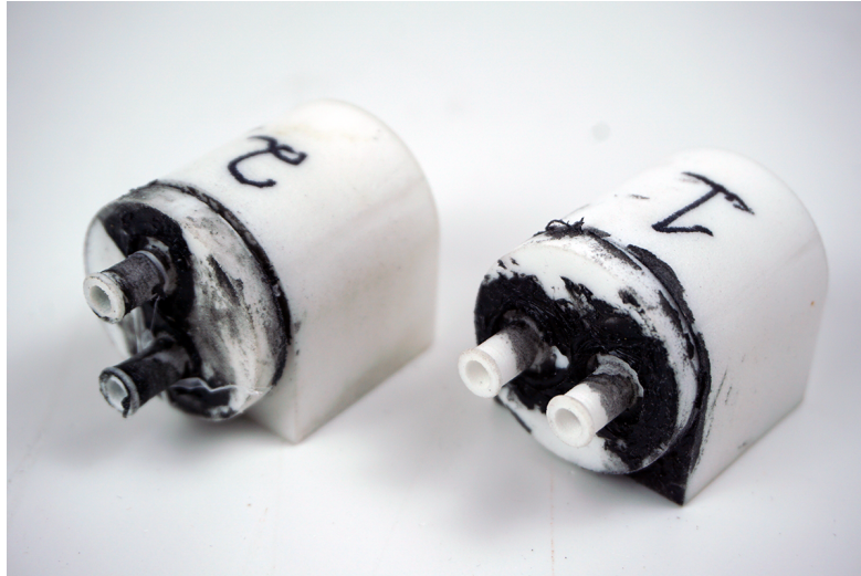
Figure 5.40: 3D print of TSI concept 3. The black splotches are silicon sealant used to waterproof the prototype
