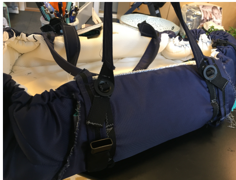
Figure 7.9: A prototype of the removable handles
