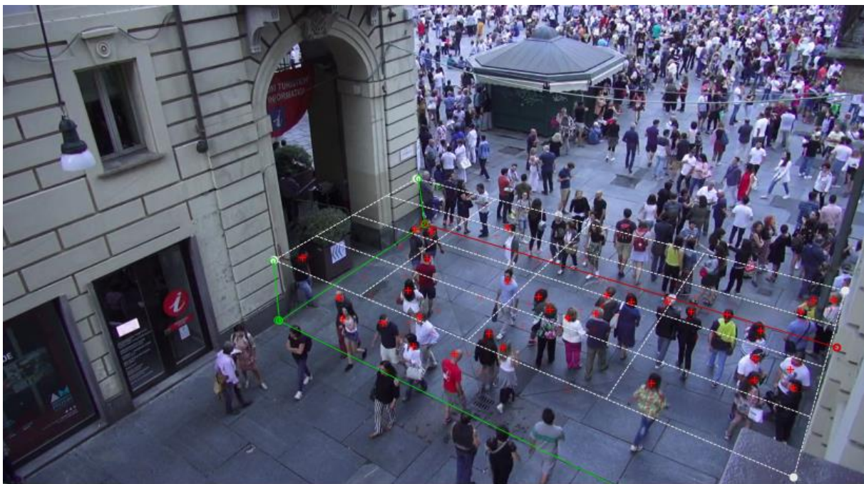
Figure 10. Definition of the control volume using a prospective grid during the stuffing phase. The dots white line in the image is the prospective grid used to easily visualise people in the area. The green solid lines have been used to build the control volume, to draw them the vanishing line of the floor have been used. The red solid line has been used to measure the flow. The red cross has been used to count the people inside the control volume.
