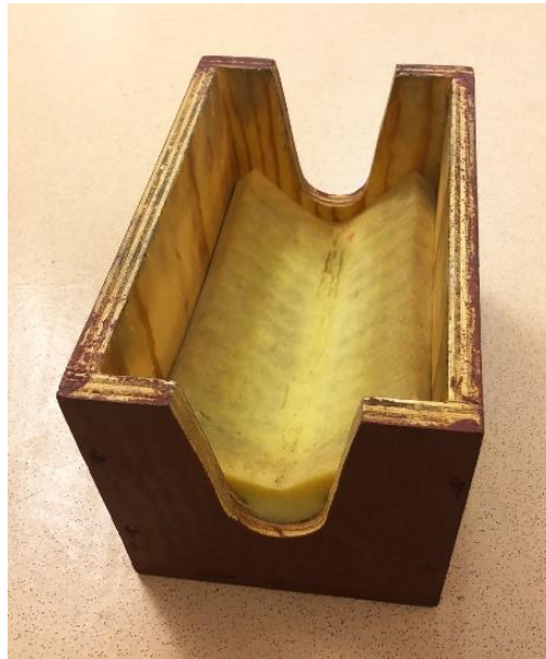
Figure 4.7: Existing solution for packaging for gear hobs (Top view).
