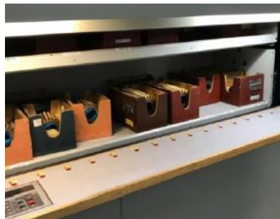
Figure 4.11: Paternoster vertical carousel in T-storage.
