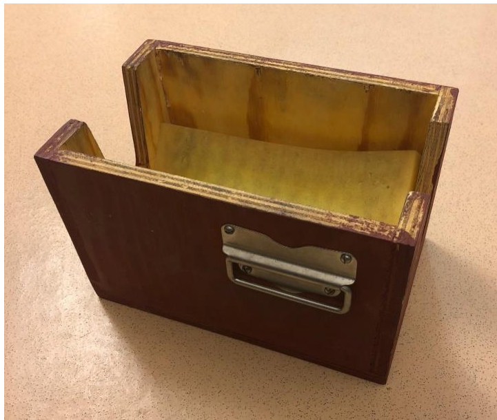
Figure 4.6: Existing solution for packaging for gear hobs (Side view).
