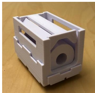
Figure 7.20: Overview of 3D printed solid model.
