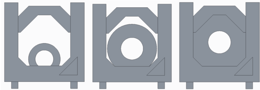
Figure F.13: Side view of short side (With gear hobs, from left: Ø70 mm, Ø110 mm & Ø145 mm).
