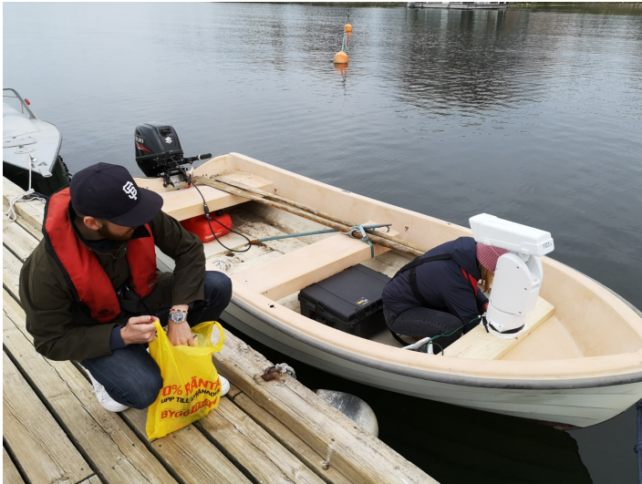
Figure 9.6: Mounting of the positioning unit on the boat.
