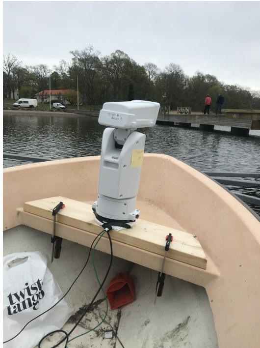
Figure 9.7: Mounting of the positioning unit on the boat, in detail.
