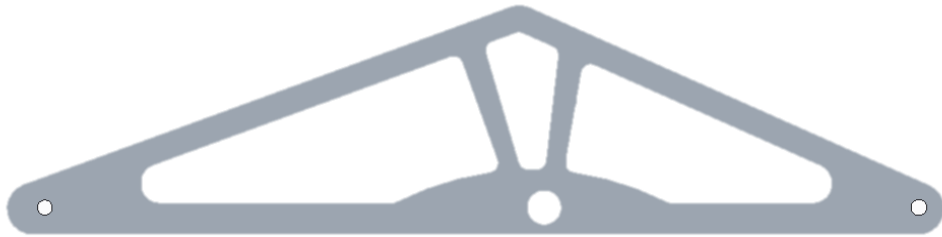
Figure 65: Redesigned structural plate.
