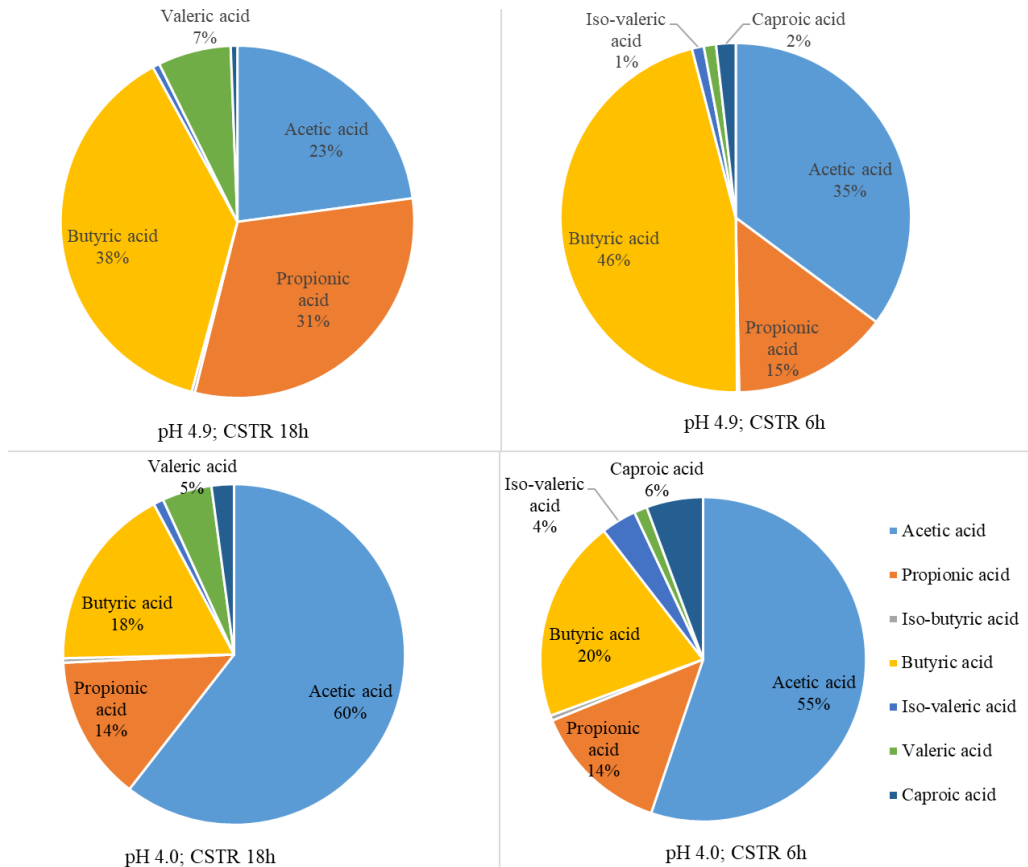
Figure 4.8 The proportion of different acids of the total VFA, under four operation conditions.
