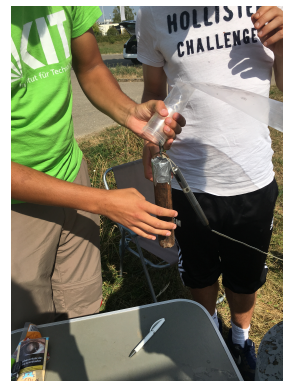
(b) A beaker, which is attached to a heavy anchor, fixed at the bottom of the plastic hose. The beaker seals the bottom of the plastic hose during preparations and before injection of salt solution application.
