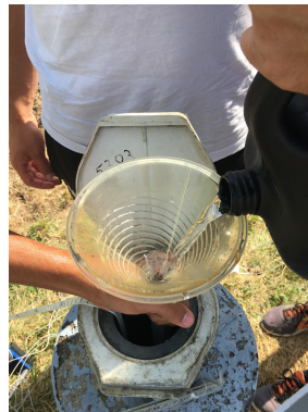
(c) Salt solution being applied into the plastic hosepipe in the borehole by using a funnel.
