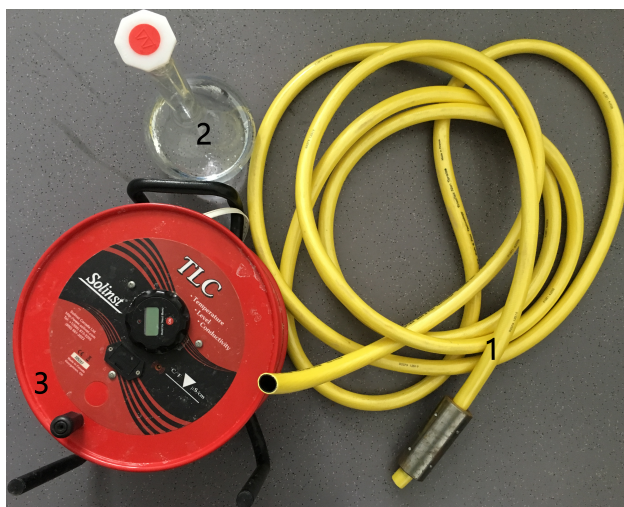
Figure 6: Setup of tools and materials used in a SBDT performed with the hosepipe method (type 2).
