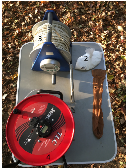
Figure 3: Setup of tools and material used in a SBDT performed with the stocking method.
